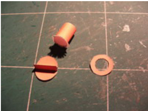
Cut, fold and glue items 21, 22 and 23 as above. make sure that the assembly will be able to go into item 15 with ease.
