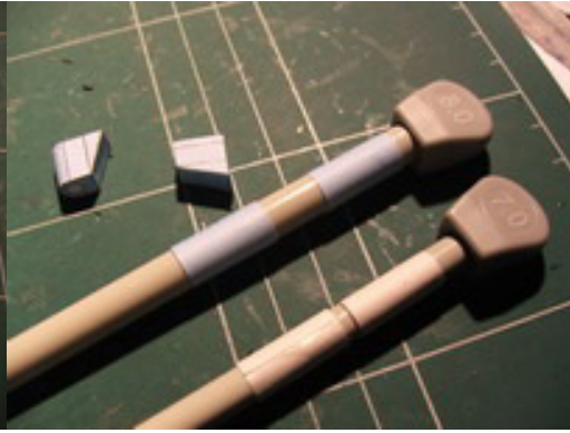
fold, roll and glue item 18 as above. Roll item 43 around a 8mm needle, roll item 44 around 7mm needle.
