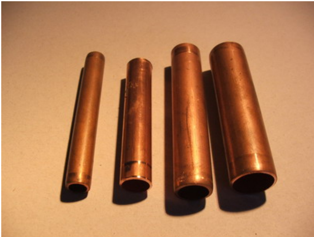
One can use plumbing brass pipes for larger parts, in this case the 12, 15, 18 and 22mm copper pipes are shown above.
