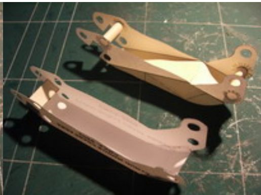
Now glue the two assemblies as above together, make sure that they all line up.
