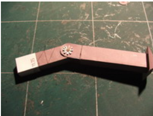
Place item 38 into items 40 and 29 then glue again carefully as for movement.
