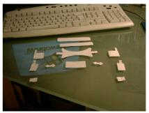
Glue the supporter to its crossbeam. (same method like coupling) (left pic) Then glue the junction plates. Glue the baseplates to the smaller feet.
