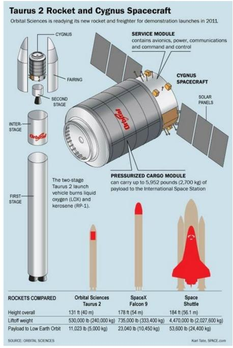
The Taurus II is Orbital Sciences Corporation's rocket for the NASA commercial orbital transportation services contract (COTS) to resupply the International Space Station (ISS). Taurus II is a two stage rocket. The first stage uses two Aerojet AJ-26-62 engines, burning kerosene and liquid oxygen, based on a Soviet design for their N-1 moon rocket. The second stage is encapsulated below the fairing and is an ATK Castor-30A solid rocket motor.
