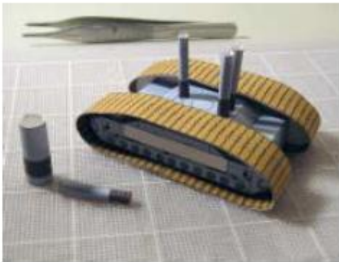
Photos show the guiding tube and cylinders in their corresponding places. IMPORTANT: Let the tubes dry well before gluing it to the crawler's corner.
